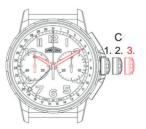
Note: do not forget to push the crown "C" back to its winding position 1 when you have set it, to guarantee the water-resistance of your watch.
