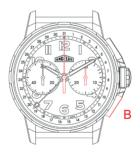
Once the timing operation has been stopped, the two chronograph hands can be reset to zero by pressing pusher "B". The chronograph is then ready for a new timing operation.
