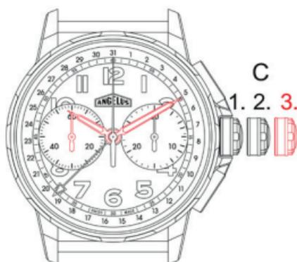
Note: do not forget to push the crown "C" back to its winding position 1 when you have set it, to guarantee the water-resistance of your watch.
