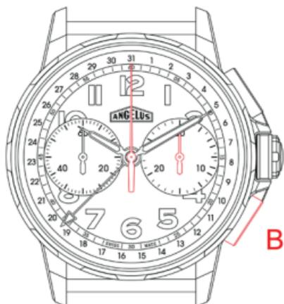
Once the timing operation has been stopped, the two chronograph hands can be reset to zero by pressing pusher "B". The chronograph is then ready for a new timing operation.
